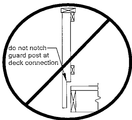
FIGURE 28: NOTCHING AT GUARD POSTS
